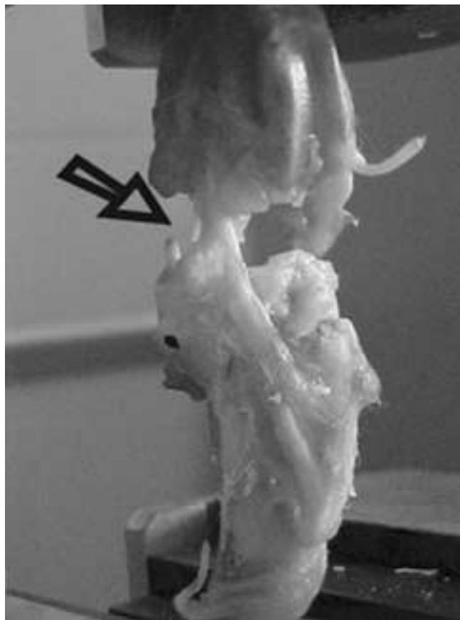
**Figure 1.** Uniaxial tensile testing of the rat MCL (arrow) with the knee in extension.
